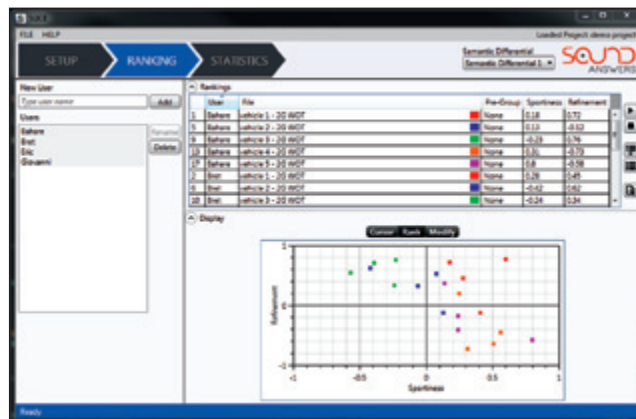
Figure 3. SLICE application used for visualizing metrics; plot shows subjective rankings of sportiness vs refinement.
