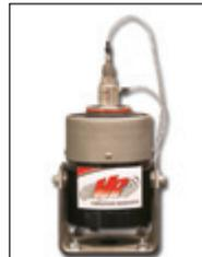
Turn-key system performs calibration verification on all sensors in your lab. System performs a sine sweep, controlling on a reference accelerometer, then automatically calculates accelerometer sensitivity at chosen frequency. Variety of customizable report templates. High-frequency for sine recommended for sensors rated > 4,900 Hz.
