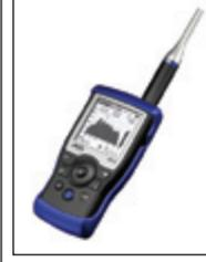
Adding the Spectral Limits option to the NTI XL2 acoustic analyzer adds an ISO 1/6 and 1/12 octave RTA function and supports all standard international standards for noise curve measurements in rooms. (NC, NR, etc). The XL2 then shows the noise spectrum mapped onto the appropriate limiting noise curve number.
