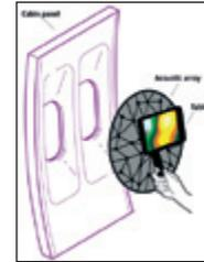
Brüel & Kjær's new PULSE Reflex Acoustic Camera is a complete kit for real-time noise source identification and data recording, designed to be up and running in 20 seconds. Making it easy to identify and measure non-stationary noise events in areas such as aircraft cabins, cargo bays, and passenger vehicles.
