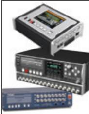
TEAC data acquisition features intuitive setup with selectable 24/16-bit resolution. Solid-state memory; DC, IEPE, video, CAN and strain inputs; analog and digital output; LAN-Ethernet interface, and multi-unit record sync. Each functions totally independently or as a front end for direct PC HDD recording. Contact: 440.935.7729 or [datarecorder@teac.com](mailto:datarecorder@teac.com)
