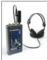
SQobold offers the utmost in portability for sound and vibration recordings and analysis; no need to lug along a tablet. Four channels of data input includes onboard GPS and video inputs for further documentation. Functions include sound level measurement and various analyses such as FFT, octave, specific loudness and sharpness versus time.
