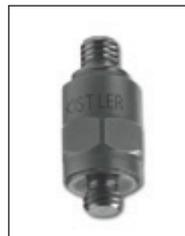
Type 8774B and 8776B families are single-axis, 3-g, ceramic-shear sensors available in many configurations to fit most modal and vibration applications. Integral stud or ground isolated, adhesive mount, top or side connector, integral IP 68 cable configuration for underwater; g ranges from 50 - 500 g available.
