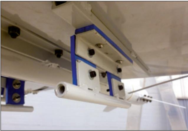
Figure 19. Damping material used to attach payloads to wings at hard points.
