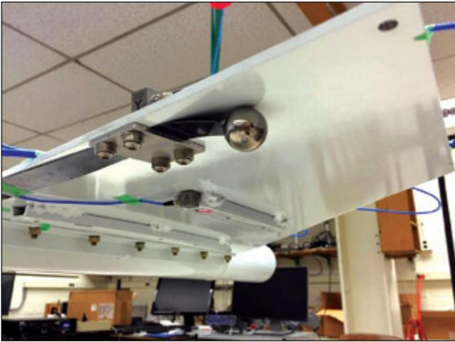
Figure 20. Flexure used to approximate aileron flutter.
