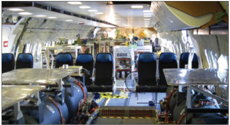
Figure 1. Typical commercial airliner outfitted for flight testing.
