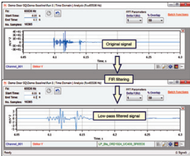
Figure 5. Time-domain presentations of original response (top) along with the corresponding low-pass filtered response (bottom) for car door closing.
