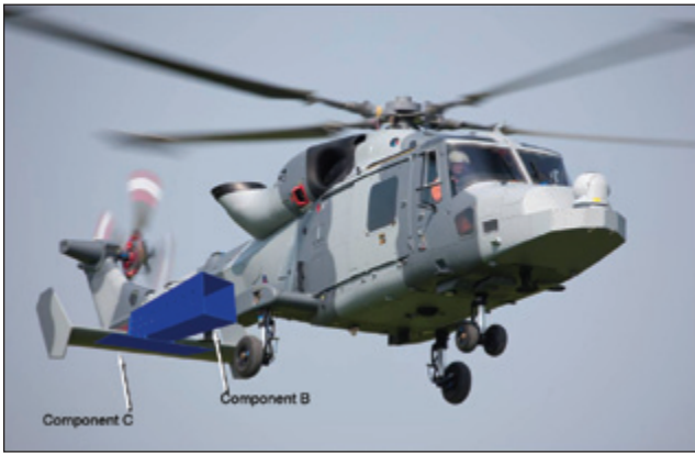
Figure 5. Composite photograph showing inspiration for the UB100X structure – the AgustaWestland 159 “Wildcat” tail cone and wing.
