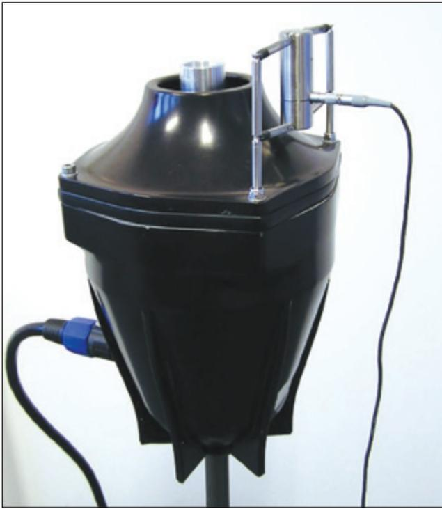
Figure 3. High-sound-level monopole loudspeaker.
