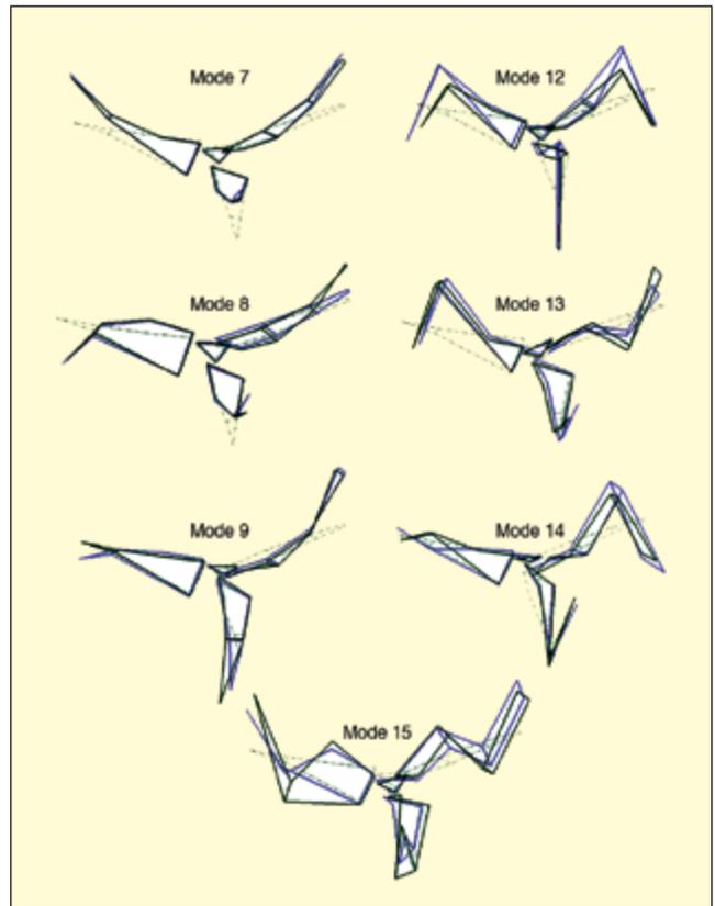
Figure 5. Bending mode shapes comparison: blue - substructuring prediction; green - truth test; broken line - undeformed).
