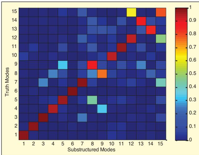
Figure 4. Modal assurance criterion between truth test and substructured predictions; first six modes are rigid-body modes (Modes 7 - 15 shown in Table 1).
