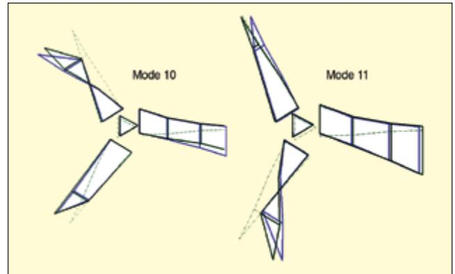
Figure 6. Torsion mode shapes comparison: blue - substructuring prediction; green - truth test, broken line - undeformed).
