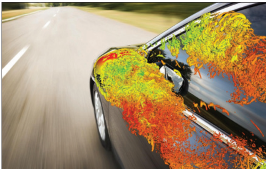
Figure 1. Fluctuating surface pressures on side glass of car calculated using OpenFOAM®, open-source CFD code. Complex, fluctuating surface pressure data can be imported into VA One from nearly any commercial CFD code.
