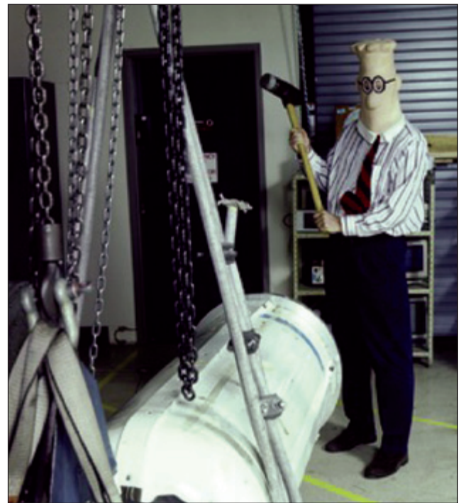
Figure 3a. Impact test on missile hung at locations close to the nodes of the first bending modes.
