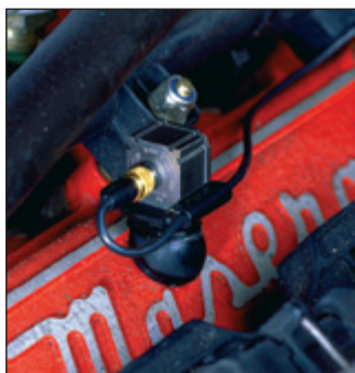
Figure 7. The 4506 triaxial accelerometer mounted on swivel base.
