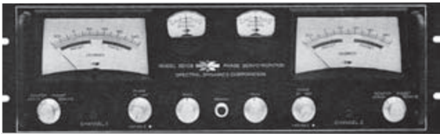
Figure 8. SD108 Phase Servo Monitor.
