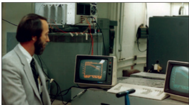
Figure 45. SD1700 Javelin controller on shaker controlling its own 6 g_{rms} test as Tom Fielder looks on.
