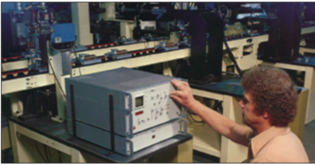
Figure 40. SD210A Spectratester on a production line.
