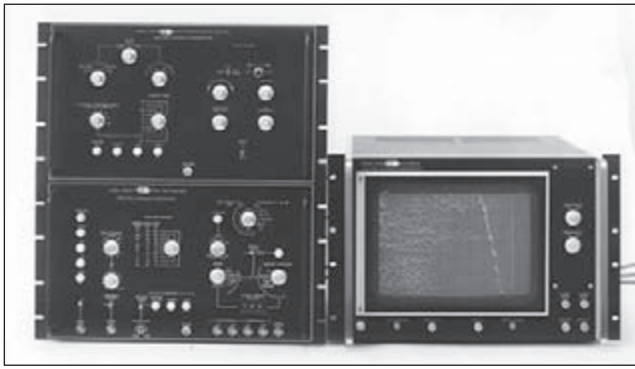
Figure 18. Spectrogram Display Control – the first “digital waterfall.”
