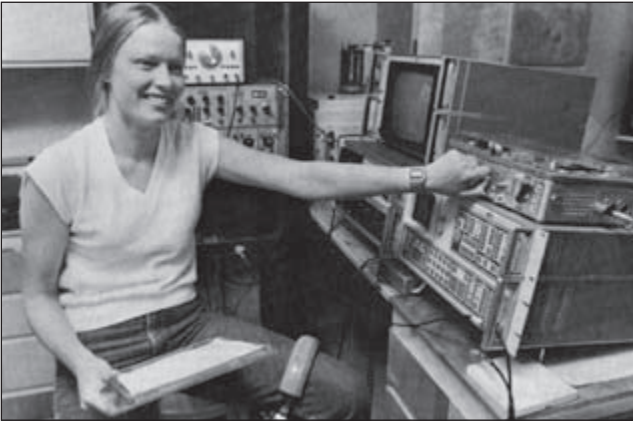
Figure 41. Jeanette Thomas at work in the HUBBS-Sea World Research Institute acoustic lab – one of the most sophisticated of its kind in the country. Below her left hand is one of the lab's key instruments – an SD345 Spectrascope III.
