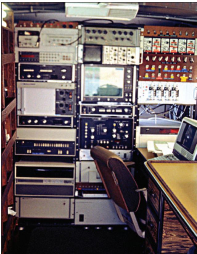
Figure 3. Analysis van – inside view of instrumentation; note the real-time frequency analyzer and plotter similar to those shown in Figure 2.
