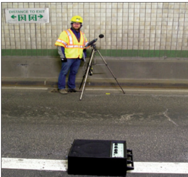
Figure 9. Reverberation time test (Site 2).
