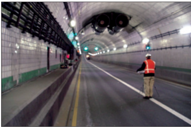
Figure 4. Jet fan 8 noise measurements (Site 4).
