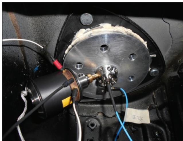
Figure 18. Inertia shaker attached to stiff aluminum plate glued to the original top-strut mount.
