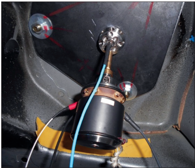
Figure 5. LMS Qsources integral shaker with 3D adapter at front top strut mount location.
