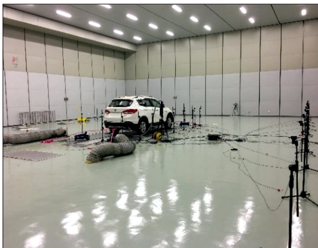
Figure 2. Site layout of indoor pass-by noise test.
