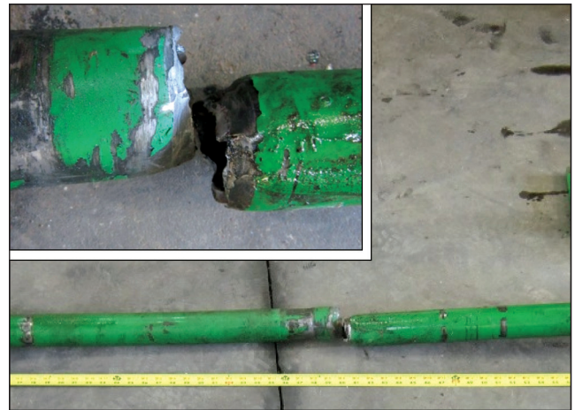
Figure 1. Critical speed failure of driveshaft that resulted in buckling failure.
