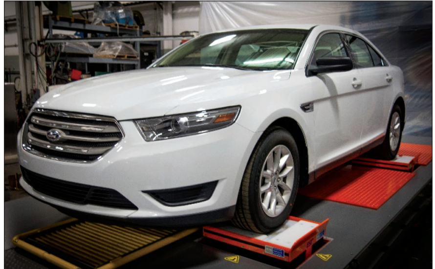
Figure 1. Four-post shaker system with full vehicle under test.
