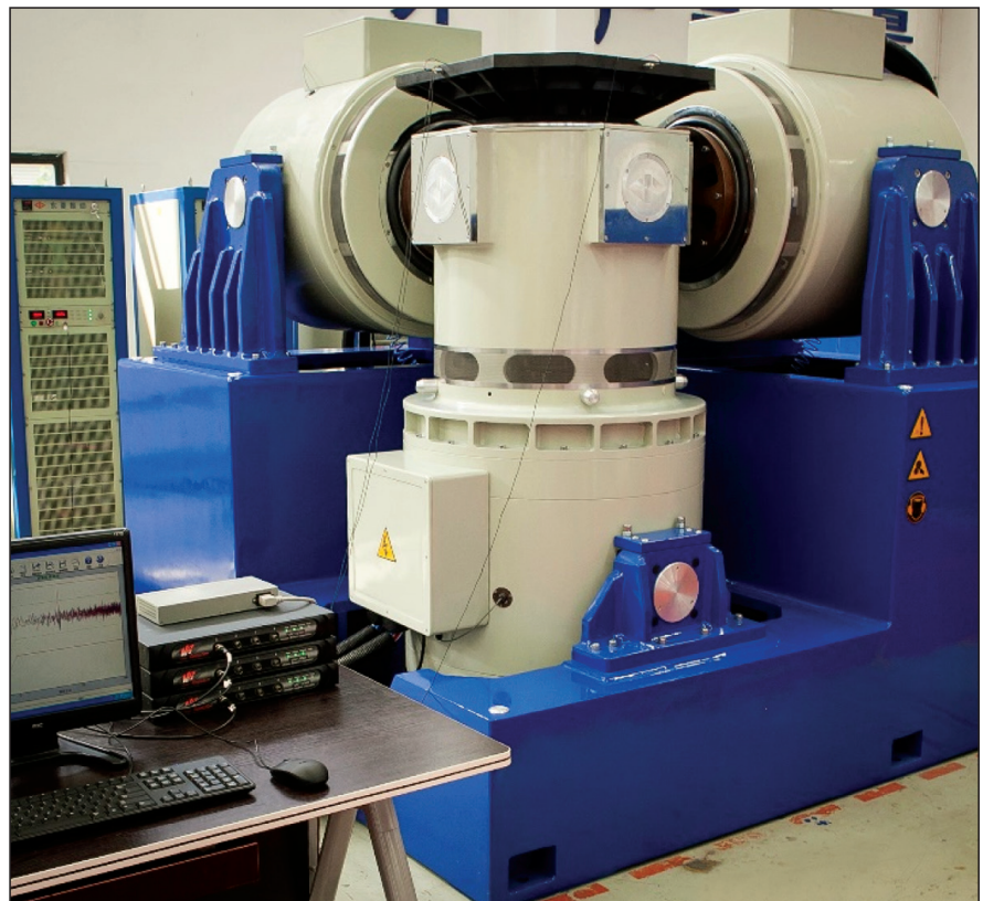
Figure 2. Three-axis shaker system with table.
