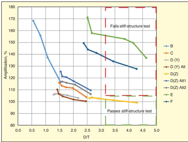
Figure 4. Pulse amplification and stiff structure test.
