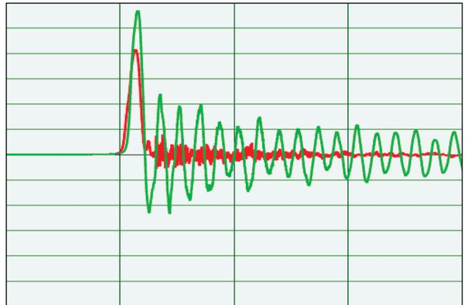
Figure 3. Table (red) and Fixture B (green) measured acceleration; duration at table – 0.37 msec.
