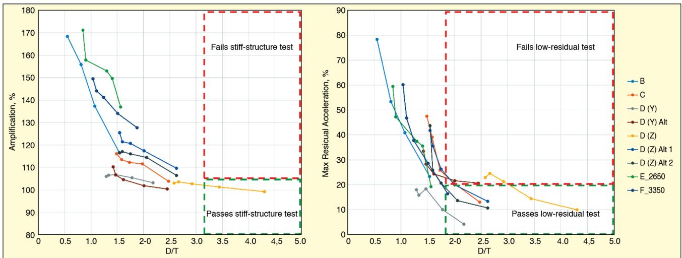
Figure 6. Amplification and residual acceleration with D/T adjusted on fixtures D and E.
