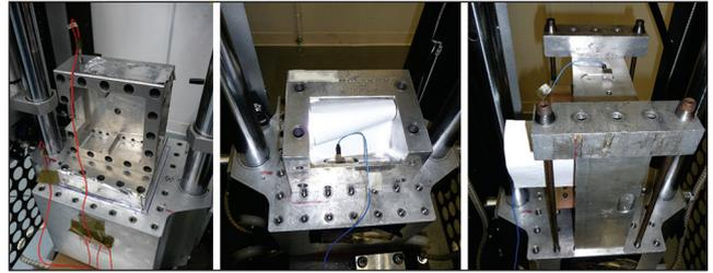
Figure 1. Fixture B with adapter plate, fixture D(Y), fixture E with straps.
