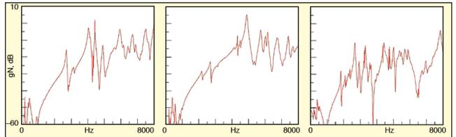
Figure 2. Driving-point FRFs for fixture D(Y), D(Y)alt, and fixture E.
