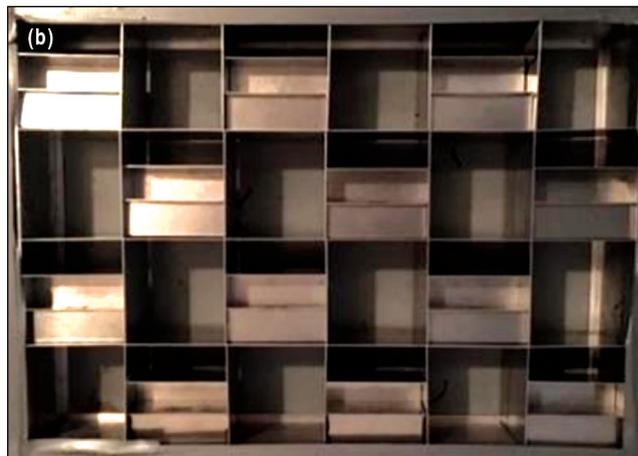
Figure 9. Three-channel backings installed behind MPP: (a) cells fully populated with backings; (b) alternating cells with backings.
