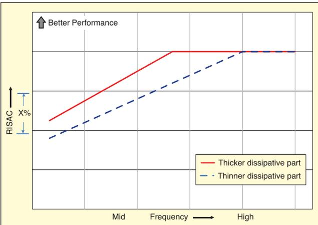
Figure 4. In-vehicle performance prediction using IL and absorption data.
