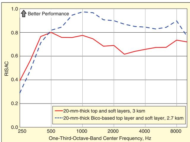
Figure 7. Effect of Bico on acoustic performance.
