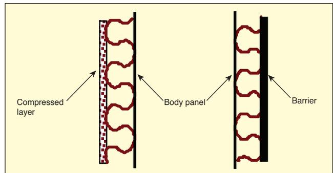
Figure 2. Schematic of dissipative and barrier decoupler system.
