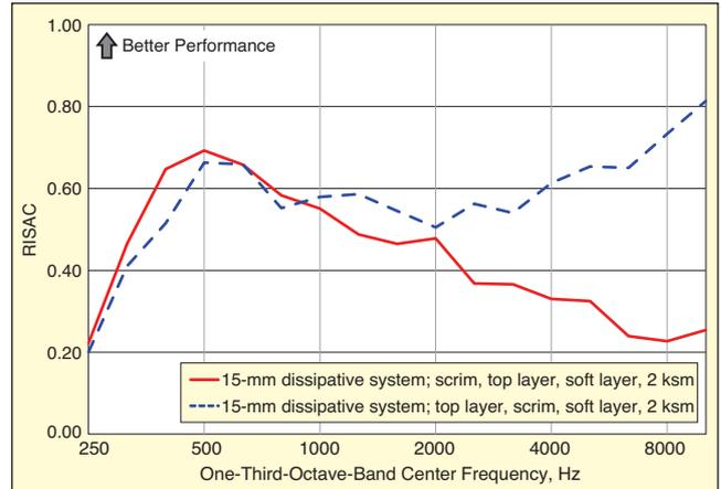
Figure 11. Effect of placement of scrim on sound absorption coefficient.
