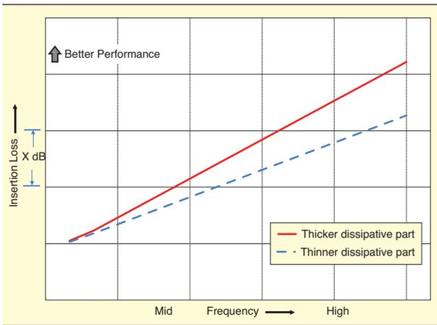
Figure 3. Typical absorption curve in specification for dissipative part.
