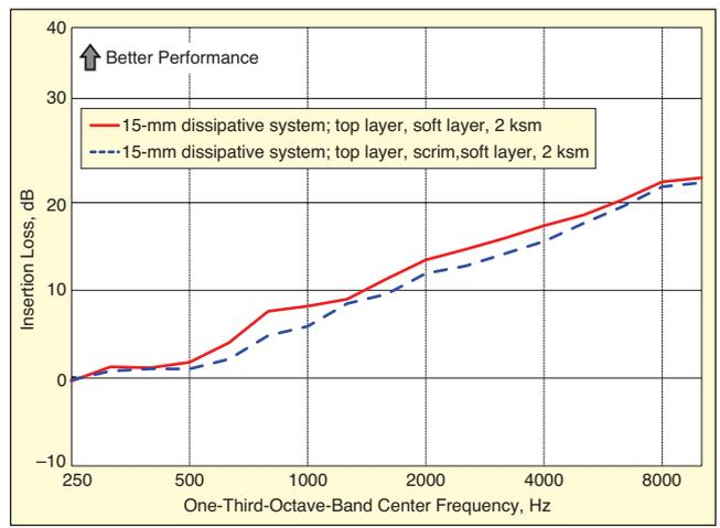
Figure 10. Effect of placement of scrim on insertion loss.
