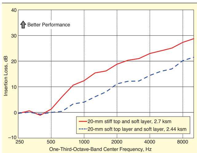
Figure 8. Impact of stiffness of compressed layer on insertion loss.
