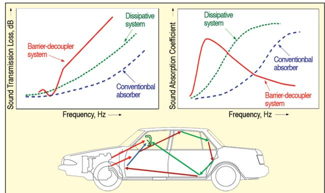
Figure 1. Typical acoustic performance of dissipative and barrier decoupler systems.
