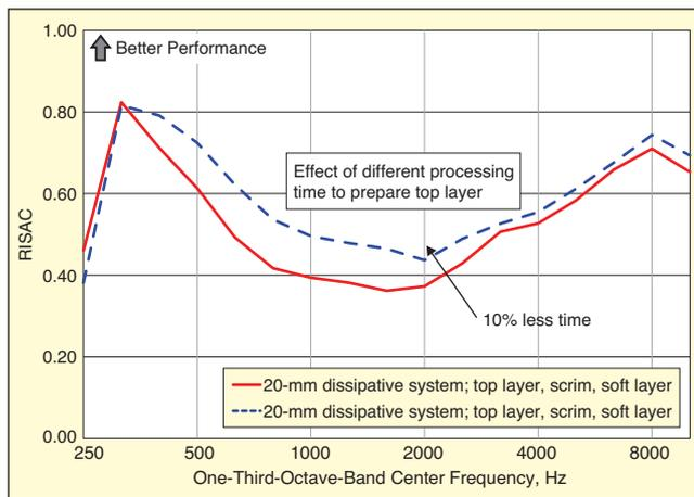
Figure 12. Impact of press time on absorption coefficient to make compressed layer.
