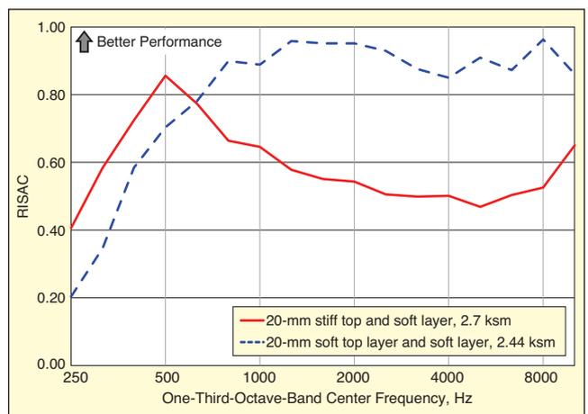
Figure 9. Impact of stiffness of compressed layer on absorption coefficient.
