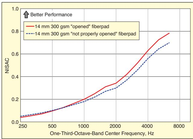
Figure 6. Impact of proper opening of fiber.
