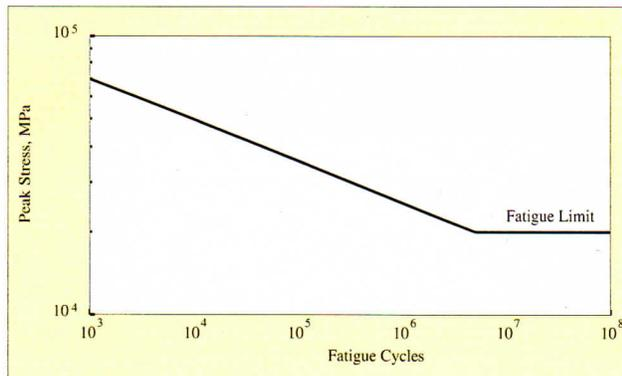
Figure 1. Idealized S-N curve for typical aluminum alloy.
