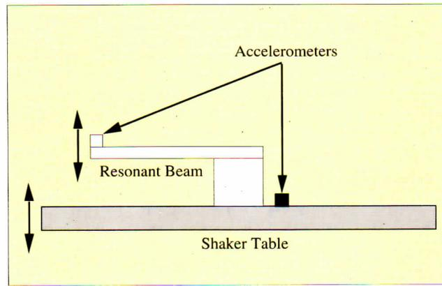
Figure 2. Test setup for a repetitive shock shaker vibration experiment.
