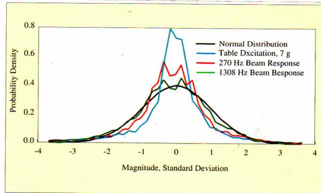
Figure 3. Normalized probability density functions for a repetitive shock shaker vibration experiment.
