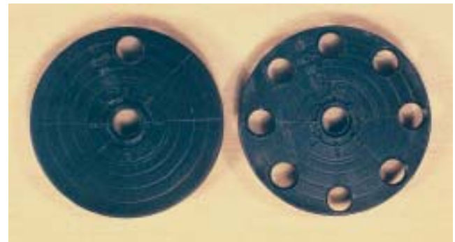
Figure 16. Two tachometer wheels used in rig testing. The wheel on the left provided one pulse per output-shaft rotation while that on the right provided eight. Seemingly minor machining imperfections degraded analysis when the 8/rev unit was employed. This is a common problem in “home grown” multi-pulse per revolution tachometers.
