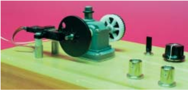
Figure 11. Gearmotor in test fixture. PCB 352C67 accelerometer monitors case vibration over the worm gear end of the transfer-shaft. Omron EE-SPX301 IR diode/receiver monitors output shaft speed, viewing disk with one or eight holes. Other sensors measure motor-current, radial magnetic flux and local sound pressure. Variable speed operation in both directions is accommodated.
