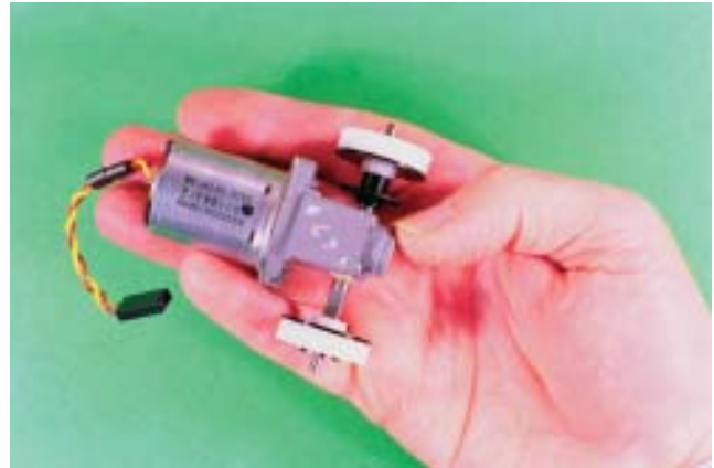
Figure 1: Our test object is the drive mechanism for a currency bill exchanger, a two-stage 36.8:1 reduction gear-train powered by a small DC motor.
